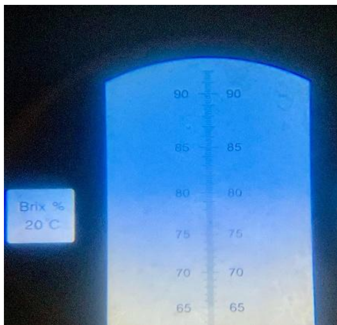
Figure 1: Measurement of °Brix value of the gummy formulation using a handheld refractometer
